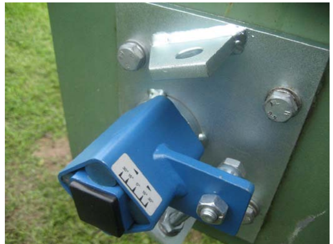
Figure 2, elastic support for primary or drum scrapers
